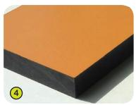
**4- Signs** are made with a compact material 13mm thick. It is made up of 70% of softwood fibres and 30% of thermosetting resin, and it stands up to weathering very well (sun, rain, damp, etc.). The coloured surfaces are treated with products based on coloured acrylic polyurethane resins; this enables them to stand up well to UV radiation and resist damage.
