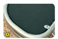
**4- The "Durax" platform floors** are machined from 22mm plywood panels made up of fine layers of birch. The surface is coated with a non-slip thermoplastic polyolefin film, and circled with a 40mm diameter stainless steel tube.
