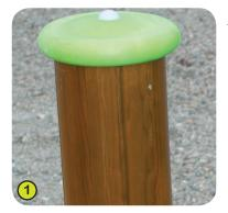
1- The 125mm round posts are made of laminated timber, which have not been treated with chrome or arsenic. Splinter-free, the laminate provides great strength and dimensional stability. The posts are protected from wear and tear caused by fungi, insects and termites.
