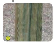
1- The 68mm square posts of the drawbridge are made of laminated timber, which have not been treated with chrome or arsenic. Splinter-free, the laminate provides great strength and dimensional stability. The posts are protected from wear and tear caused by fungi, insects and termites.
