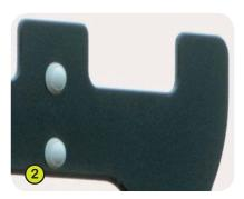
2- The painted panels are 22mm thick and made up of layers of very high quality birch which are waterproofed with a coat of phenolic resin. The edges are then sealed and 3 coats of polyurethane paint are automatically applied to each face and edge.
