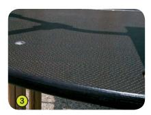
**3- The platforms** are 22mm thick panels made up of alternating layers of birch and pine. The surface is coated with a film of anti-slip phenolic resin.
