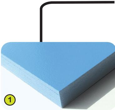
1- **The lacquered panels** are made from very high quality plywood 21mm thick, made of alternate layers of thin birch, which offers longevity and an exceptional mechanical strength. The colours are applied by electrostatic spraying of two-component polyurethane lacquer that is free of heavy metals, to ensure high levels of resistance to potentially aggressive chemicals such as anti-graffiti cleaning products.
