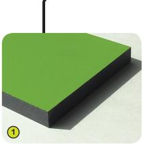
1- The coloured panels are made with a compact material 13mm thick. It is made up of 70% of softwood fibres and 30% of thermosetting resin, and it stands up to weathering very well (sun, rain, damp, etc.). The coloured surfaces are treated with products based on coloured acrylic polyurethane resins; this enables them to stand up well to UV radiation and resist damage.
