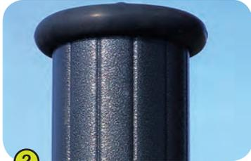
2- **The 125mm diameter posts and the 95mm square posts** are made of lacquered galvanised steel. The two-tone grey graining finish has a slightly undulating surface for increased scratch resistance. The caps are made of injection moulded polyamide.
