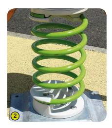
2- The springs are made from Grade 35SCD6 steel, shot blasted, stress relieved, zinc coated and finished with two coats of epoxy polyester powder. Proludic have patented an exceptionally strong and secure polyamide fixing for the spring, ensuring a long product life.
